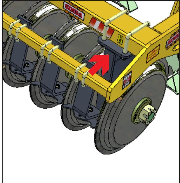
Fig. 5.02: DD Roll Grease Points
