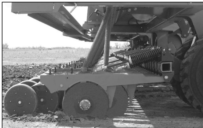
Figure 55 Frame & Openers Level
