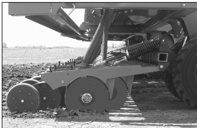
Figure 56 Openers Too High in Front
