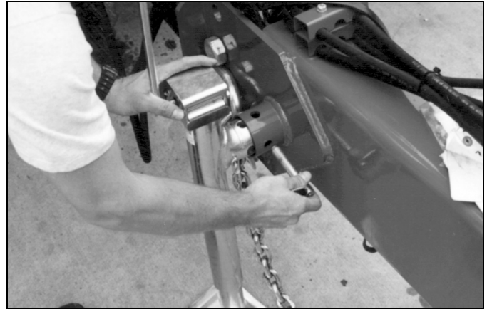
Figure 4 Jack in Lifting Location
