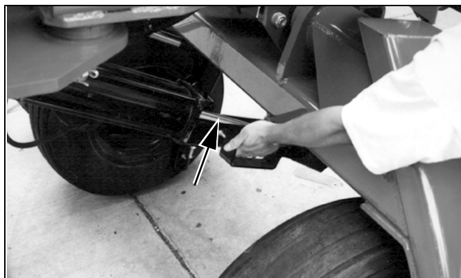
Figure 19 - Fold Transport Lift Cylinder Lock
