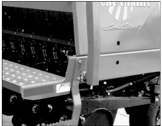
Figure 42 Wing Stand Pinned Up
