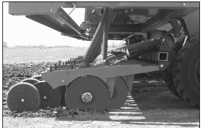
Figure 45 Openers Too High in Front
