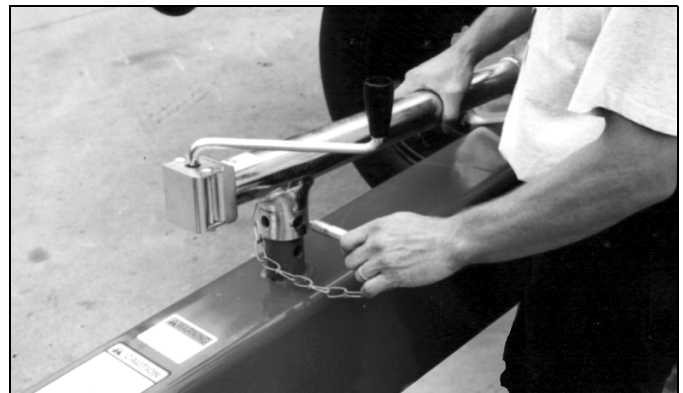
Figure 6 Jack in Storage Location
