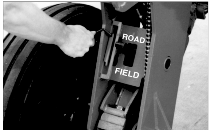
Figure 16 - Fold Opener Lock Up
