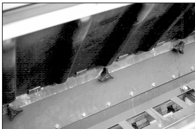
Figure 32 Seed/Fertilizer Flap Closed
