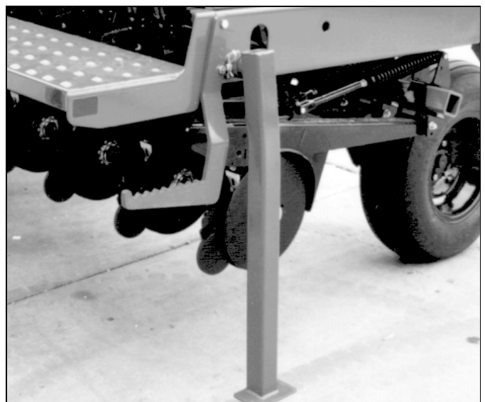
Figure 43 Wing Stand Pinned Down
