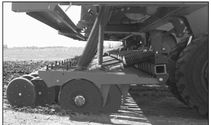
Figure 46 Openers Too Low in Front
