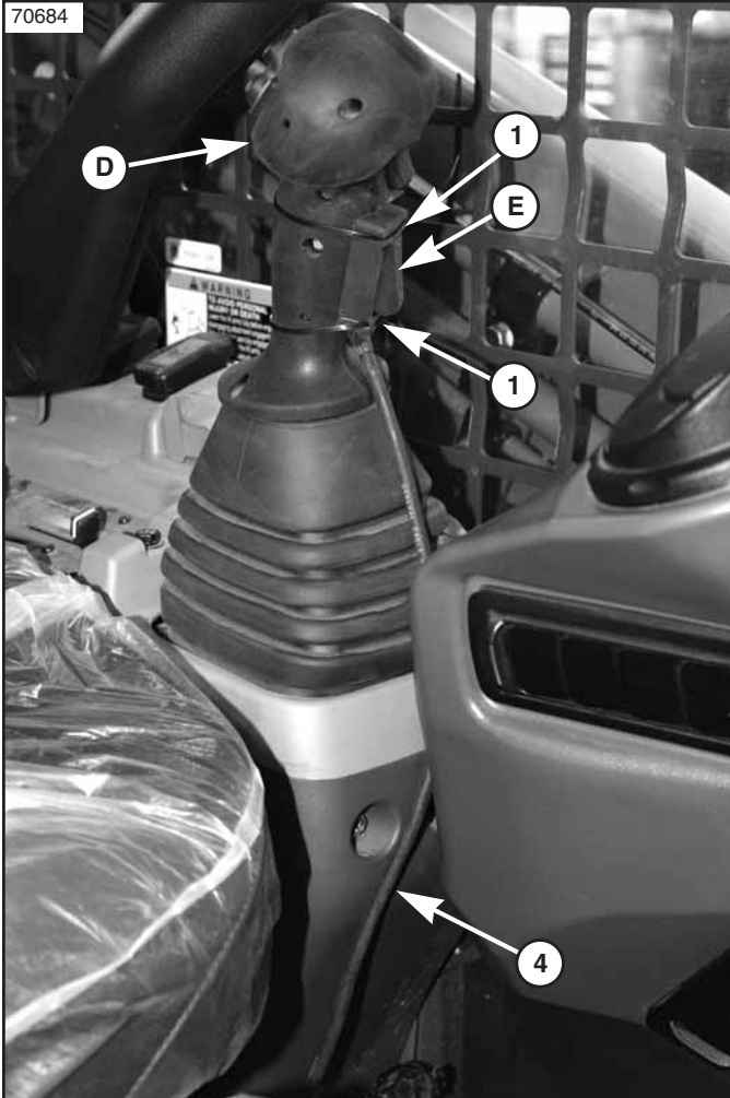
Mount Momentary Switch to Control Lever Figure 11
