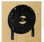
10 Gauge stump jumper is backed with a 1" x 4-1/2" thick blade mounting bar to protect the gearbox seal and output shaft.
