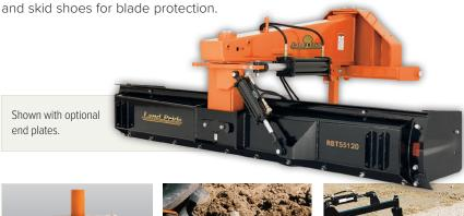
Pivot weldment features a 1" thick plate steel turntable, 3/4" thick tilt pivot bushing and a 4" solid kingpin.
