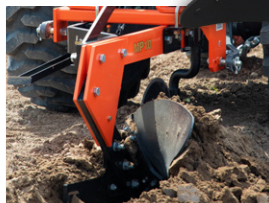
Replaceable shares, shins, and landsides offer easy maintenance.
